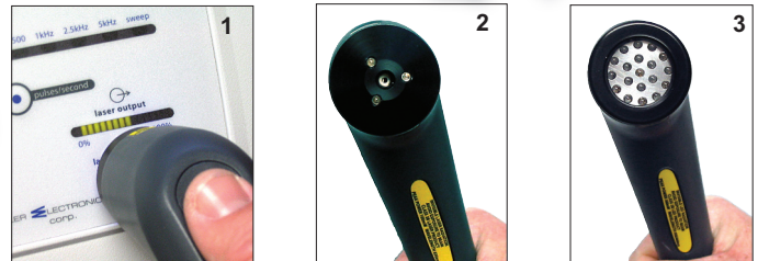
(1) laser applicator over laser output sensor showing visible proof of laser activity; (2) laser applicator showing one laser diode at 785 nm surround by 3 LEDs at 470nm; (3) cluster applicator showing 12 SLDs at 950 nm with seven LEDs at 660 nm
