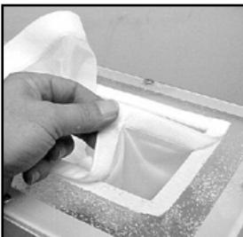
Carefully pull the hook and loop fasteners apart to remove the sleeve from the unit.
