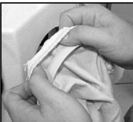
Remove the ring from the folded end of the sleeve.
