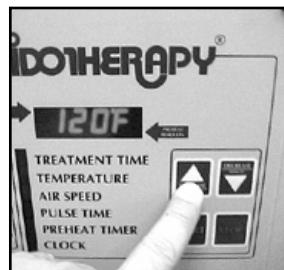
Press the "INCREASE" and "DECREASE" buttons to set unit to the desired default treatment temperature.
