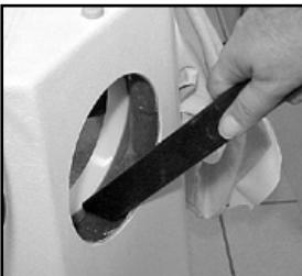
Vacuum out any of the Cellex medium that may have entered the cavity between the inner and outer walls of the unit.
