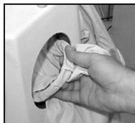
Pull the sleeve away from the sleeve extrusion in the inner housing of the unit.
