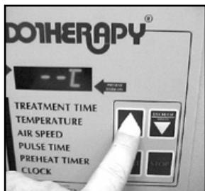
Press the "INCREASE" button to set unit to display °F or °C as desired for the default setting.
