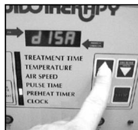
Press the "INCREASE" button to set unit to display "EnAb" or "dISA" as desired.
