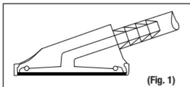
For low-frequency response (bell phase) simply hold the chestpiece in place with light pressure. (Fig. 1)
