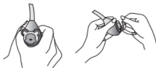
**Replace:** Position the bottom of the new plate to the socket of the chestpiece. Snap the top firmly into place.
