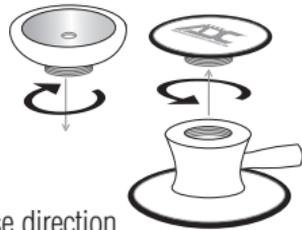
To remove pediatric diaphragm, twist in a counterclockwise direction.
