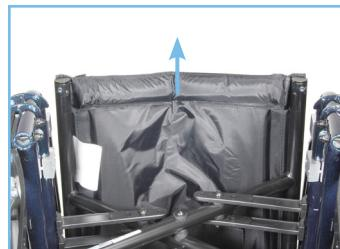
1. Lay wheelchair on its back. Open seat two-thirds of the way so seat posts do NOT rest on chair frame. Unfold seat extension by pulling upward on end of seat to release hook and loop fastener.
