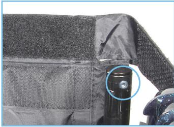
3. The seat extension post is located inside the seat frame. To access it, turn screw counter-clockwise and remove it.
