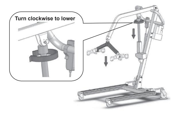
The device consists of a plastic collar ring that should be turned clockwise continually until the patient has been lowered.
