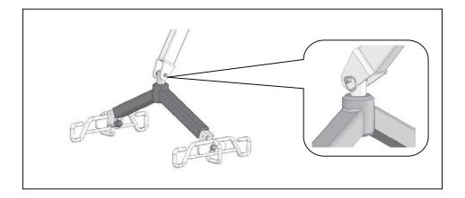
9. Attach the spreader bar bracket to the boom and insert retainer pin, as shown above. Insert retaining ring through retainer pin to secure spreader bar to boom.
