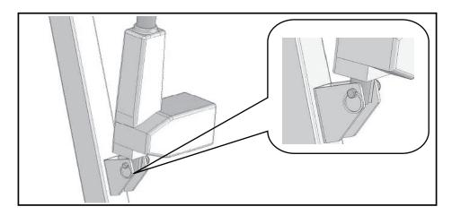
7. Attach the actuator bottom to the mast bracket and insert retainer pin, as shown above. Insert retaining ring through retainer pin hole to secure actuator base to mast bracket.
