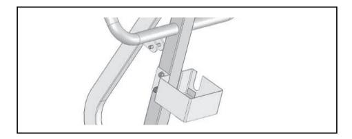
5. Attach the control box hanging bracket to the mast, as shown above. Tighten the nuts.
