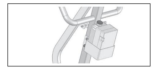
6. Place the control box in the bracket, as shown above.
