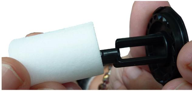
Fig. 4 - 8 Top of filter element holder removed
