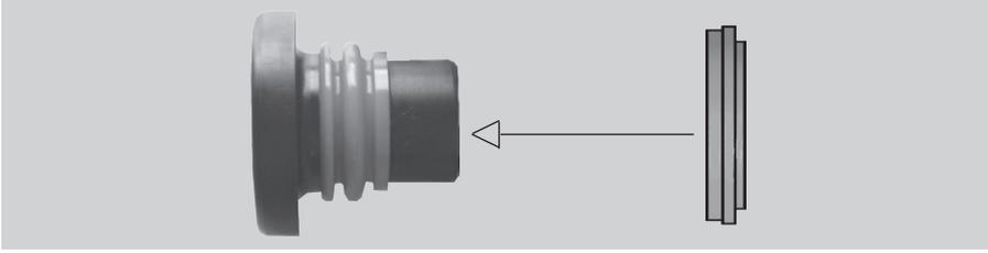
Fig. 9 - 6 Mount the sealing ring
