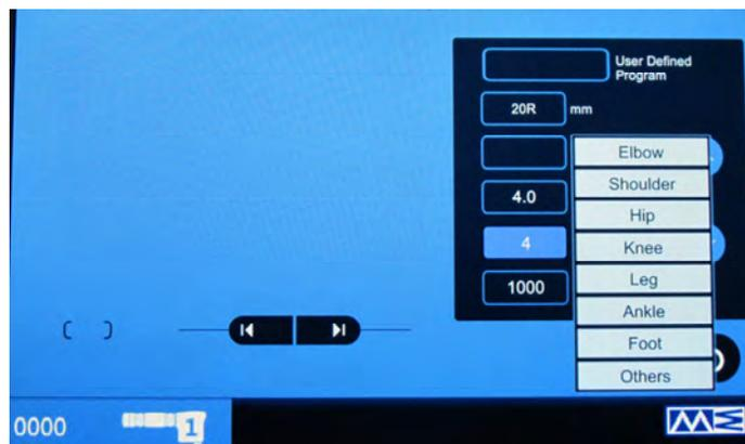
STEP 6: Set treatment parameters: pressure, frequency, and number of shocks. (You can adjust them by touching the **UP** and **DOWN** button in the right-hand side of it.)
