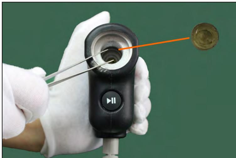
**Step 3:** Put a new spacer into the handpiece and make some adjustment with a tweezers. Make sure the spacer is
