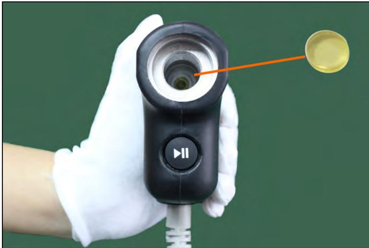
*Step 4: Reinstall the handpiece and test the performance (start the machine and listening to the sound of the handpiece)*
