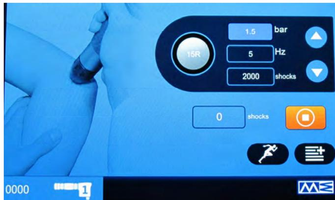
**NOTE:** Pressure and Frequency are adjustable during the treatment (Pressure adjustable with 0.1 bars; frequency adjustable with 1 Hz), while number of shocks cannot be adjustable during the treatment.
