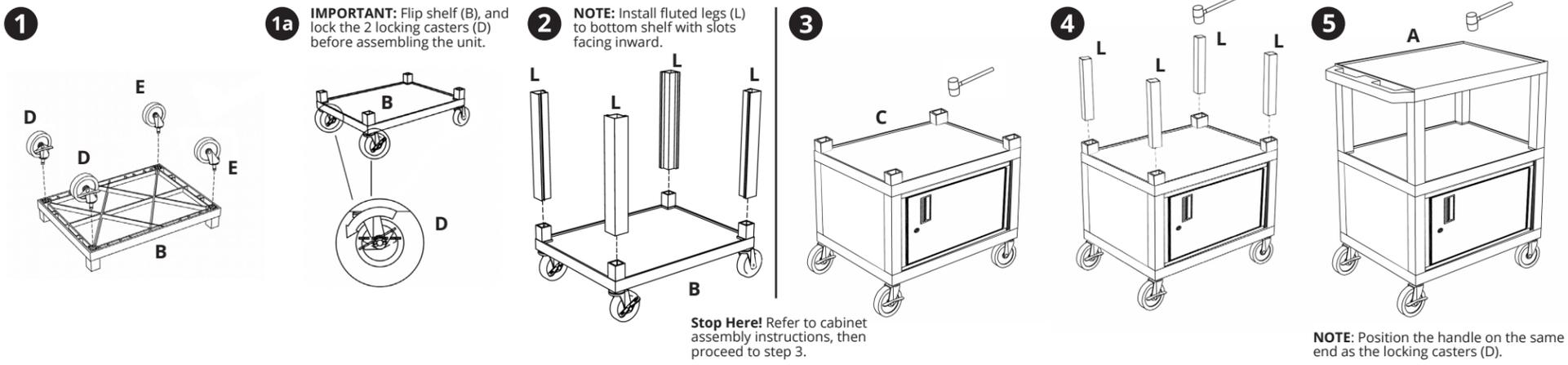
1a IMPORTANT: Flip shelf (B), and lock the 2 locking casters (D) before assembling the unit.
