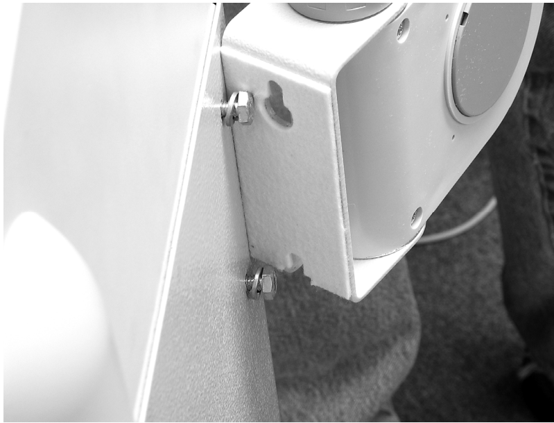
Figure 3.3—Mounting The Arm To The Cart
