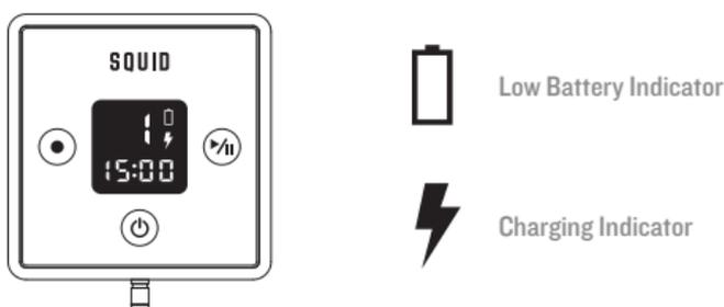
FIGURE 3 - LOW BATTERY & CHARGING INDICATORS
