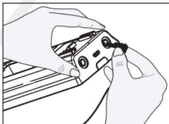
**Note:** If you use only one Channel, only plug in 1 lead wire at the top of the unit
