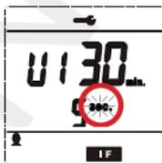
After you have finished with the settings, press the [ **⏻** ] button to confirm, the device will go back to the home screen.
