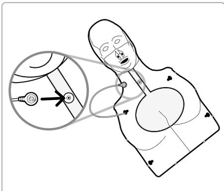
4) Attach the Breath module to the breath module holder situated on the lung bag. Put back the skin of the manikin and make sure the lung bag is not strangely folded.
