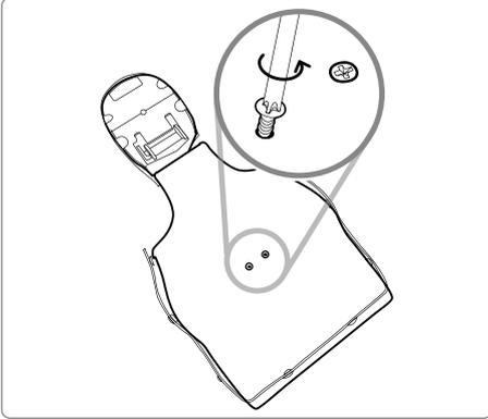
1) Disassemble two screws from the back of the manikin. If the screws are not installed on your version please proceed to the next step.
