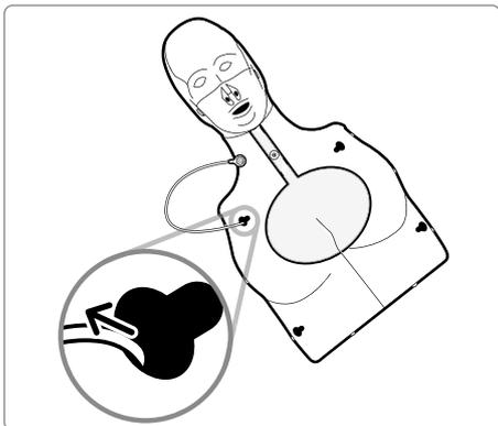
3) When assembling chest frame back to the manikin, do not forget to pass the breath module through the left top hole on the chest frame
