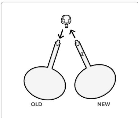
2) Remove the lung bag which is not equipped with the Breath module holder and install the new lung bag delivered in the Upgrade kit.
