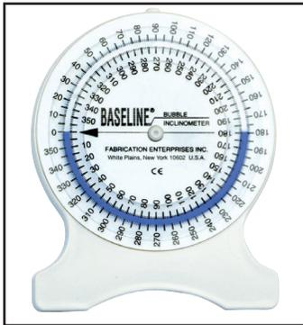
Inclinometers and goniometers are devices used to measure range-of-motion. Range-of-motion can be measured from the neutral position to give a reading of flexion, extension, abduction, adduction, pronation, supination, dorsiflexion, plantarflexion, etc. or it can measure the entire range to yield a total range-of-motion of the joint.
