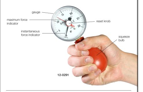
2" squeeze bulb dynamometer measures PSI.
