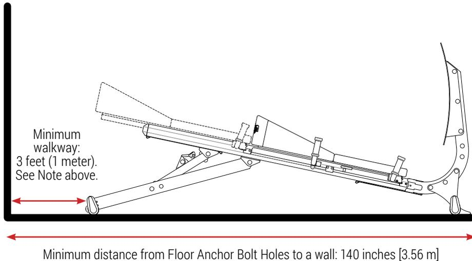
Bolt down machine at Front Base through the Bolt Holes provided on the Anchor Feet. **NOTE: INSTALLATION MUST BE CARRIED OUT BY A PROFESSIONAL INSTALLER.**
