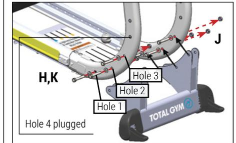
The image below is how the Front Base attached to the Struts should look.
