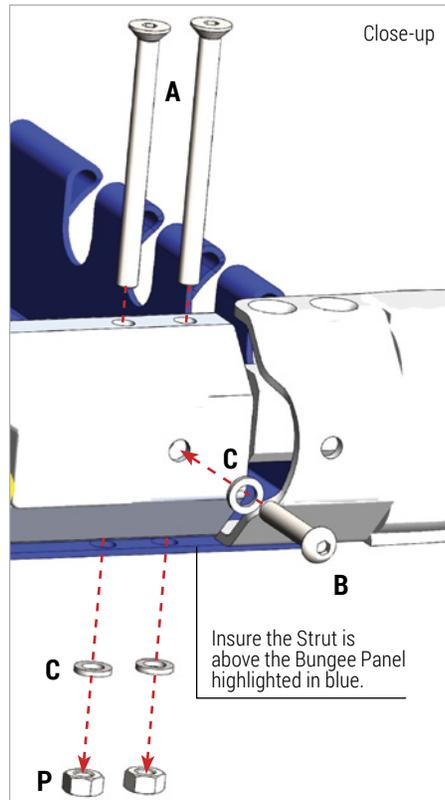
**STEP 3.** Repeat STEP 2 on other side, attaching the Right Squat Strut to the Right Rail using the hardware (A, B, C, P) as shown, but do not tighten completely.
