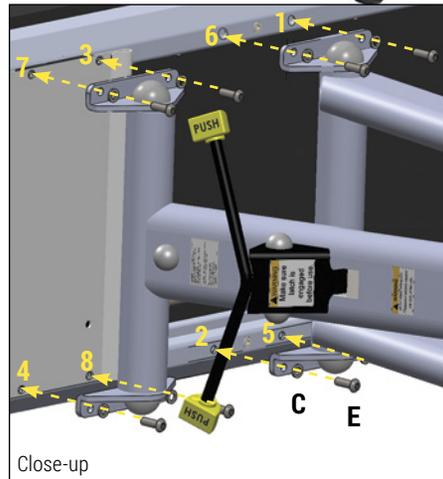
**STEP 8.** Turn the LEX upright and, using the hardware (H, J, K, S) as indicated; attach the Squat Stand to the Struts. Tighten completely. Installing the screws in the order shown may be easiest. Once screws are fully tightened, push on all 12 caps (S).
