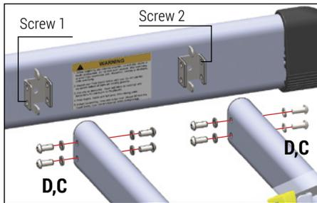
**STEP 7.** Lay the Recovery Series LEX on its side. Using the hardware (C, E) as indicated; attach the Rear Struts / Incline Strut as shown. Tighten completely.
