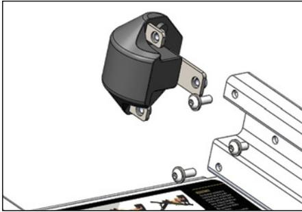
**STEP 2.** Remove the gas strut brake by unscrewing two screws below the top placard panel with a 5mm Hex wrench (Not included).
