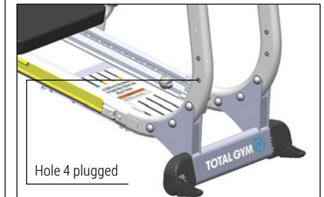
**STEP 6.** Using the hardware (D, C) as indicated; attach the Rear Base to the Rear Struts as shown below. Ensure both the logo and the warning stickers are right side up. Install screws 1 and 2 first, then proceed to install the rest; tighten completely.
