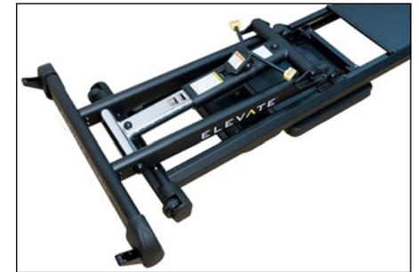
Using the 5 mm Hex Wrench, attach the hinges on to **C** with four Long M8 screws and washers. Do not tighten any completely until all four screws are installed.
