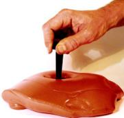
**Standard Turn:** Push base into putty, hold cap with a standard grasp, turning through putty simulating opening a bottle cap.
