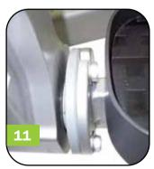
Next install a hex head bolt and washer on the right side of the disk as shown in **Figure #10**. Repeat this again on the other side of the disk as shown in **Figure #11**. There will be a total of three bolts installed.
