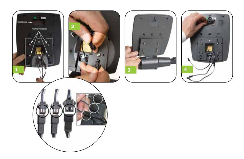
Use 4 computer bolts to secure computer to brackets. Tighten firmly but Do not over tighten. (See Figure #3)
