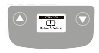
If the battery is critically low, the LCD Display Panel will show the sign on the left either when the lift is turned ON or when a button on the LCD Display Panel is pressed.
