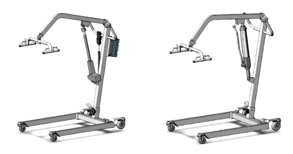
STEP 1 Install the Mast into the square sleeve located at the rear and center of the Base and tighten the black plastic hand nut by hand.
